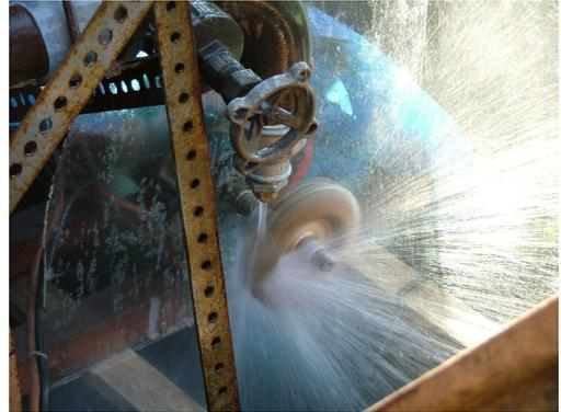
This meant we could double our head (height the water comes down from) and minimise friction losses giving us 35-40 meters of head and a possible flow much greater than previous systems due to the increased diameter of pipe used. As a result, we produced 100 watts without using much more water than on our previous system.
